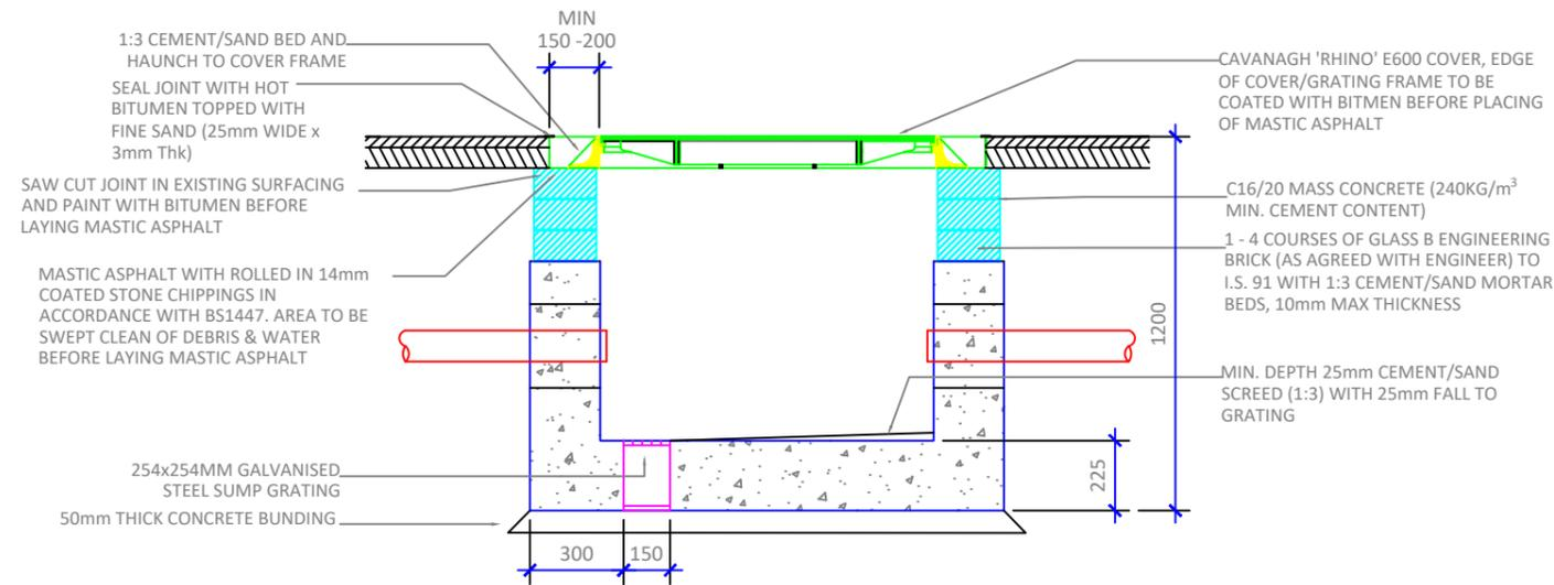
**Section Through Typical Communications Chamber**
